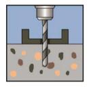
Create borehole using a Rotary Hammer
