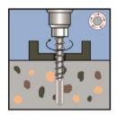
Install of the screw anchor with an impact wrench or by hand
